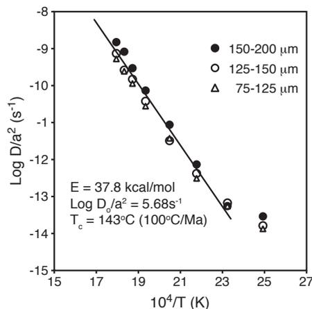
**Fig. 2.** Composite Arrhenius diagram from three size fractions. Only points representing  $^{39}\text{Ar}$  released below 300  $^\circ\text{C}$  are included.
