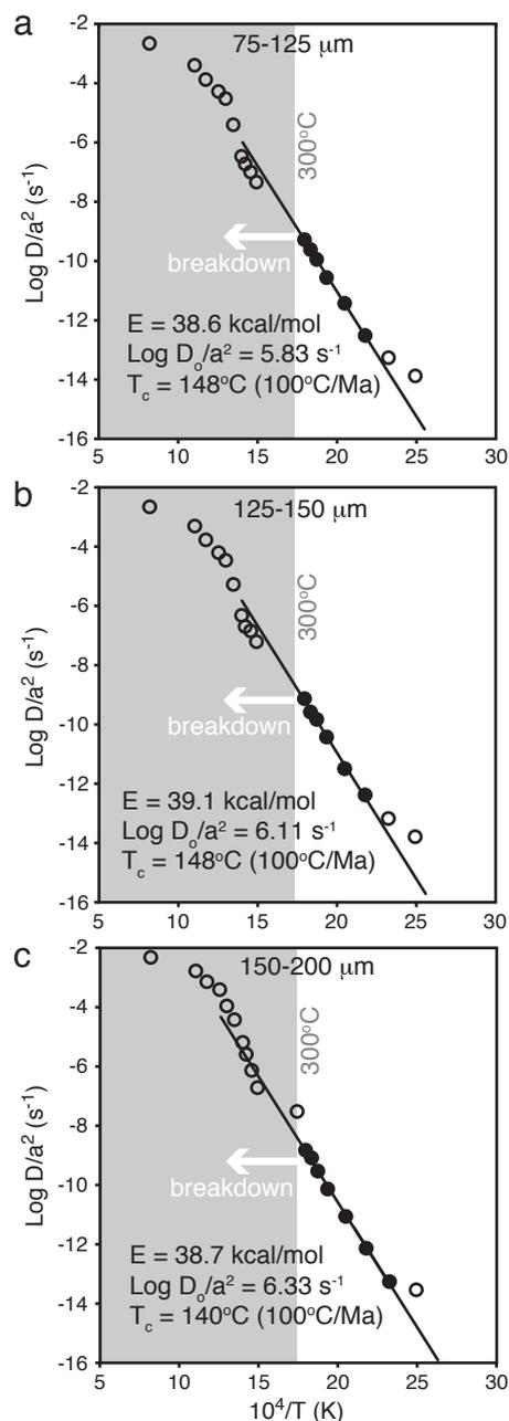
Fig. 1. Arrhenius diagrams based on incremental  $^{39}\text{Ar}$  released during step-heat experiments. a. 75–125  $\mu\text{m}$  size fraction. b. 125–150  $\mu\text{m}$  size fraction. c. 150–200  $\mu\text{m}$  size fraction. Least-square regression yields consistent results between grain sizes.
